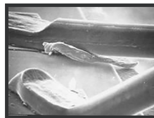
A small metal flake as shown above can cause serious malfunction in electronic components
