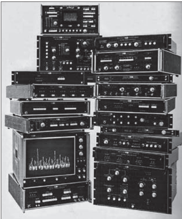
Figure 14. Some of the add-on accessories to the SD301 Real Time Analyzers. The accessories expanded the applications for the RTAs to acoustics, rotating machinery, sonar studies and much more.
