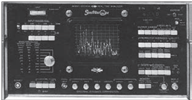
Figure 16 . The first RTA with built-in averaging and display in a single chassis.
