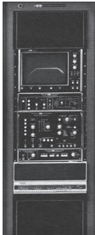
Figure 35. First SD1009A Digital Vibration Control System fed by paper tape
